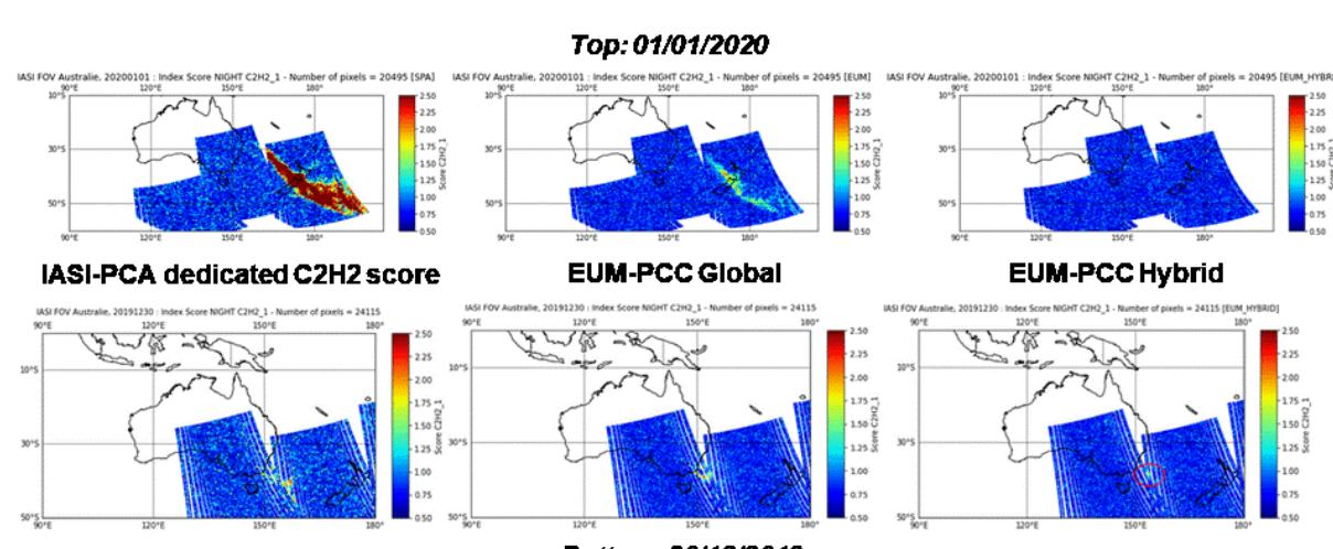
The EUM-PCC Global mode fails to reconstruct the signal for both dates (middle panel) where the IASI-PCA method detects C<sub>2</sub>H<sub>2</sub> outliers (left panel). However, the Hybrid mode is efficient to capture such rare spectral signature (right panel).
