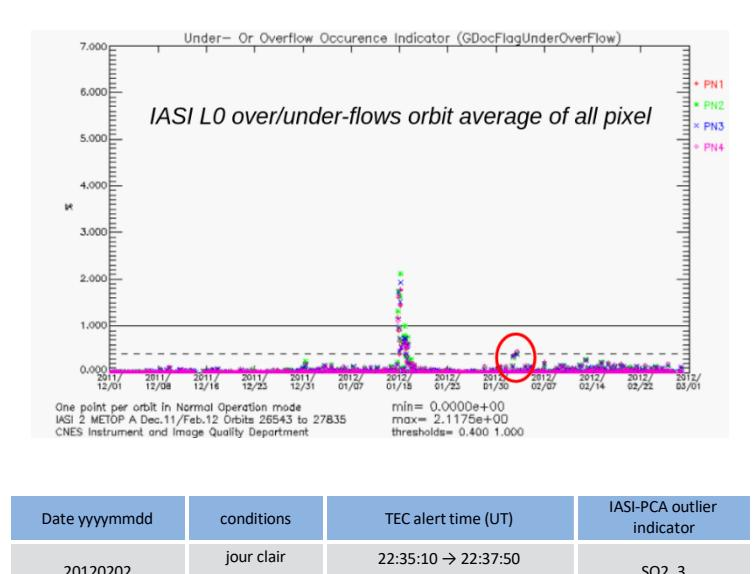
TEC under/overflow flag monitoring, and date/time of a TEC alert analysed by IASI-PCA
